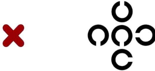
Figure 4.6: Red cross ( left ) used as initial fixation and clustered Landolt C shapes ( right ) used as target to measure vergence time. Surrounding Landolt C's pattern is used to avoid orientation discrimination using peripheral vision, ensuring correct foveation [Spiegel and Erkelens 2024].
